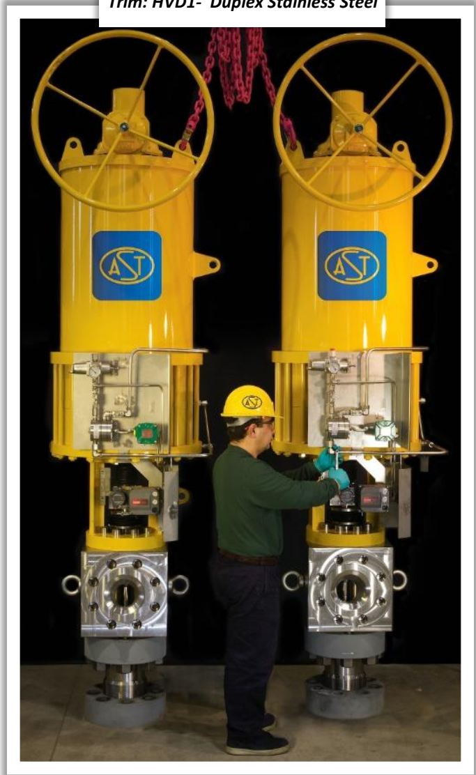
CV-870U – DN 8" PN 320 Carbammate Recirculation Body: AISI 316L Urea Grade Trim: HVD1- Duplex Stainless Steel
