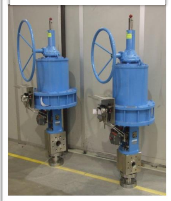
CV-870U – DN 3" PN 250 Body: AISI 316L Urea Grade Trim: UNS S32550 Duplex Stainless Steel
